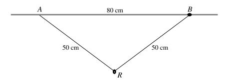
A small smooth ring R, of mass  $0.6 \,\mathrm{kg}$ , is threaded on a light inextensible string of length  $100 \,\mathrm{cm}$ . One end of the string is attached to a fixed point A. A small bead B of mass  $0.4 \,\mathrm{kg}$  is attached to the other end of the string, and is threaded on a fixed rough horizontal rod which passes through A. The system is in equilibrium with B at a distance of  $80 \,\mathrm{cm}$  from A (see diagram).
